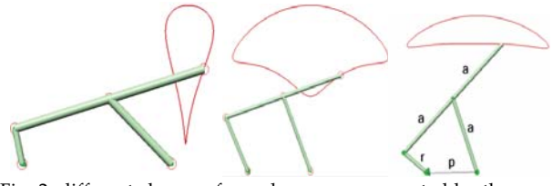
Fig. 2. different shapes of coupler curves generated by the same type of mechanism
