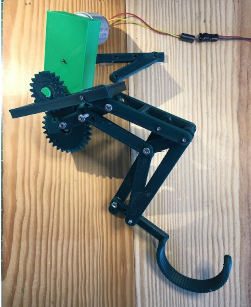
OpenSCAD - Running Robot Foot Design
