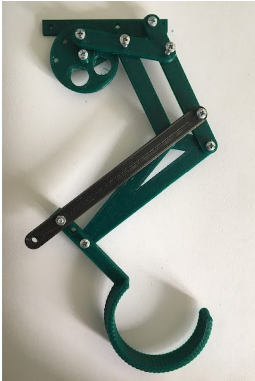
Simple Running Robot Leg Mechanism
