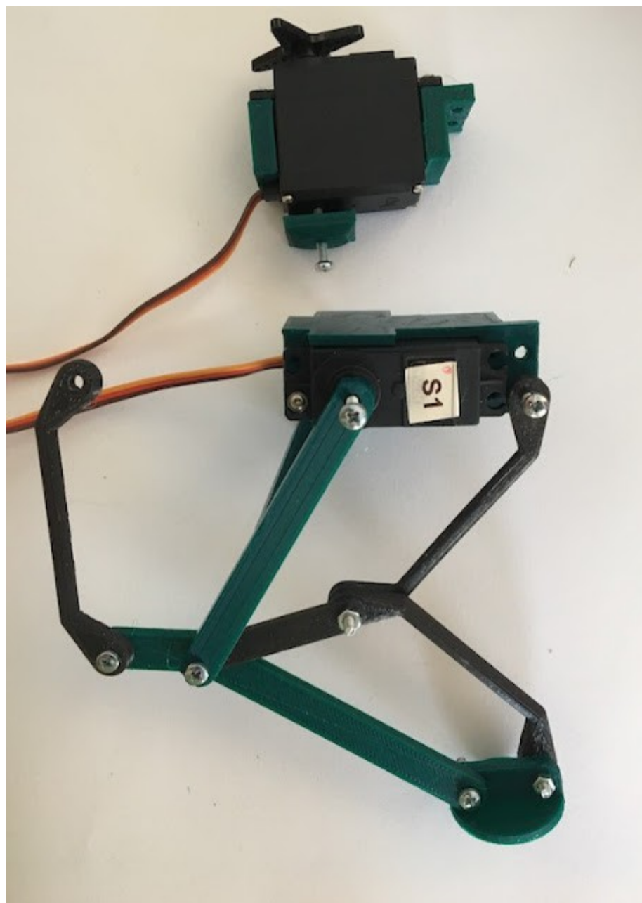
prototype-printed-sketch of a 2 dof robot leg.
