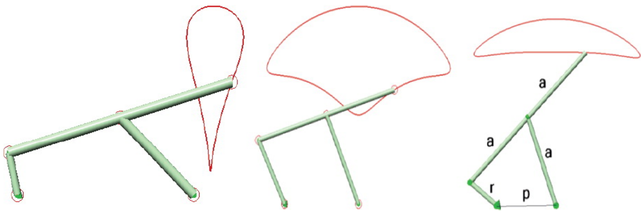
Figure 2. Different shapes of coupler curves generated by the same type of mechanism
